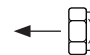
M6 nyloc nut (Always ensure nyloc nut is screwed on as shown)
