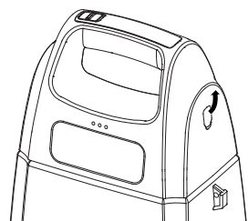
1. Remove the covering of the micro USB port.
